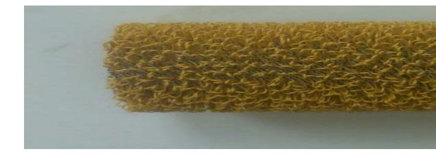
Incorrect type!! Note "compressed" loops, this will entrain air into the resin.
